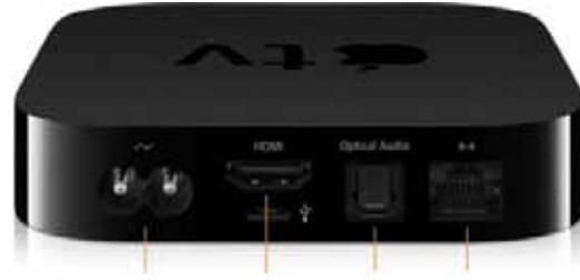
Wired ethernet is also still present, but has been reduced in speed to 100Mbps. The previous model included Gigabit ethernet to make syncing with iTunes faster, however the 2010 AppleTV no longer needs to sync anymore because it is exclusively a streaming device.
